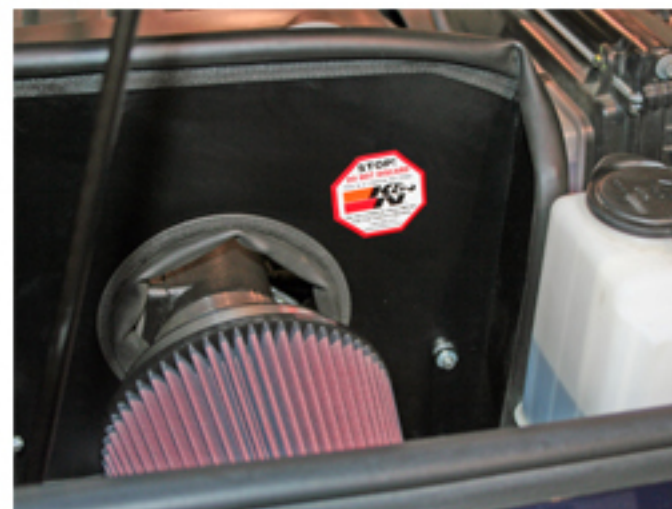
K&N air intake system 69-9031 installed on 2008 Toyota Tundra at SEMA
