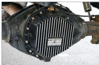
Mag-Hytec supplied the diff cover to aid in cooling, increase lube capacity...and look good.
